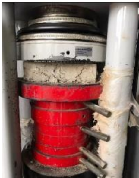
FIGURE 6. Picture of the compression test carried out.
