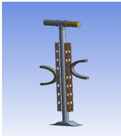
FIGURE 2 Mechanical design for force measuring device
