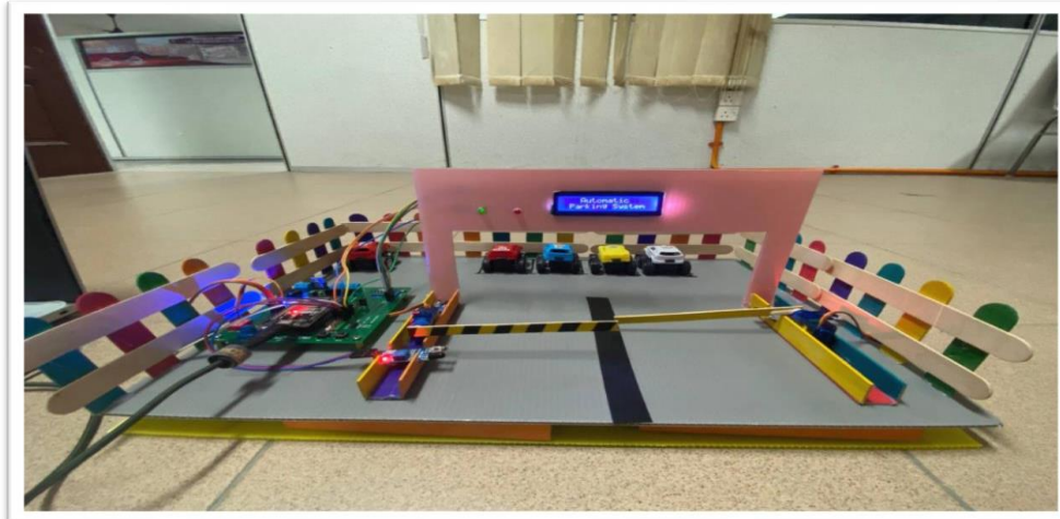
FIGURE 2. Illustrates the operational framework of an automatic parking system utilizing two infrared (IR) sensors.
